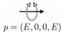
Fig. 3.4 The rotational symmetry of a massless particle. Because we cannot Lorentz boost to its rest frame, there is only one independent axis about which we can rotate.
